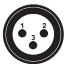
DMX-input XLR mounting-plug:
