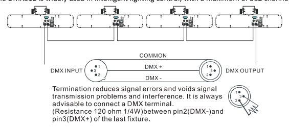
Connect the fixture together in a "daisy chain" with the XLR plug cable from the output of the
